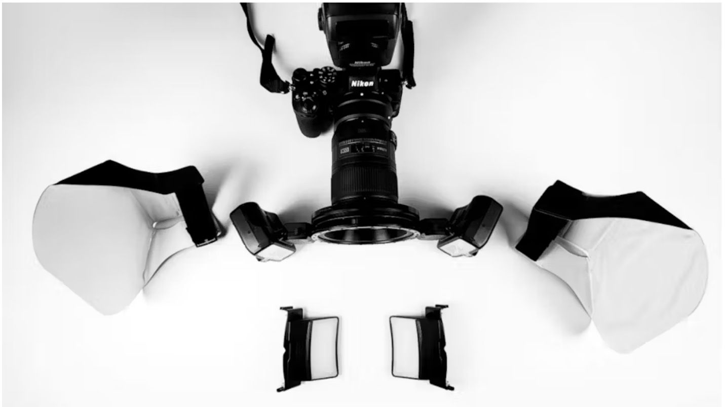
Figure 2: My third eye, MILC full frame camera with 105mm lens and various light defectors for smile ("paddles" diffusers, sides) and for posterior teeth (close-up defectors, bottom)
