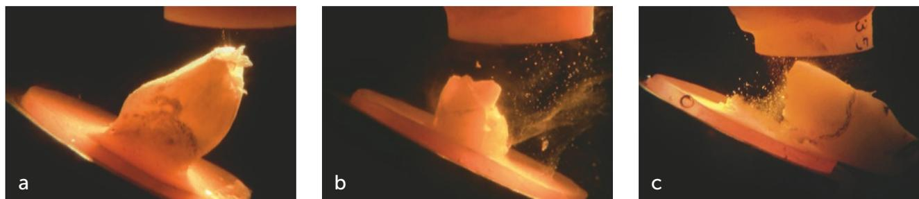
**Fig 4** Classification of failure mode of the tested specimens. Video image captured at the moment that the test finished. (a) 'Reparable' fracture (cohesive or cohesive/adhesive fracture of tooth structure or restoration). (b) 'Possibly reparable' fracture (cohesive/adhesive failure with fragment and minor damage, chip or crack of underlying tooth structure). (c) 'Catastrophic' fracture (tooth/root fracture that would require tooth extraction).
