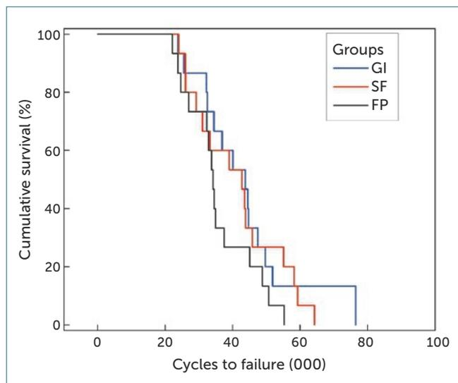
**Fig 2** Fatigue resistance survival curves (Kaplan-Meier survival estimator) for all groups. GI: glass-ionomer cement; SF: short fiber-reinforced composite resin; FP: fiber post.
