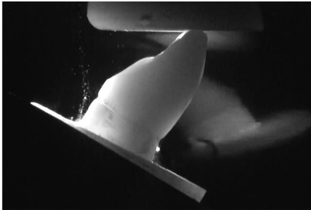
**Figure 3.** Cyclic isometric loading applied to incisal edge at an angle of 30 degrees. Initial failure as wide lingual gap between crown margin and tooth.
