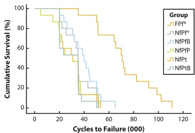
**Figure 5.** Fatigue resistance survival curves (Kaplan-Meier survival estimator) for all six groups. \*Additional groups from previously published data concomitantly tested in identical experimental conditions. B, bulk-fill composite resin core foundation restoration; F, ferrule; Nf, no ferrule; P, dual-polymerized composite resin core foundation restoration; Pf, glass-fiber post; Pt, titanium post.
