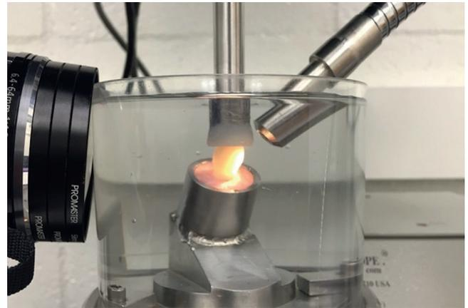
**Figure 4.** Specimen in load chamber. Macro camera and transillumination light used to identify crack propagation mode (initial and final failures).
