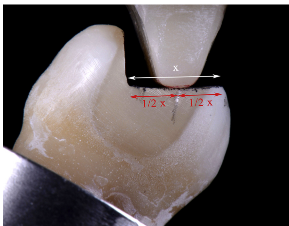
Fig. 4 – Positioning of specimen for cyclic-load-to-failure test at 30-degree angulation, and a semicylinder (2.5-mm radius) post-polymerized resin creating a single equidistant contact on the flat surface (palatal cusp).
