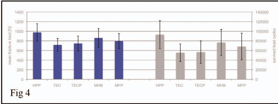
Figure 4. Mean fracture loads (blue) and average number of survived load cycles (grey) and their standard deviations, respectively (previous data included<sup>18</sup>).
