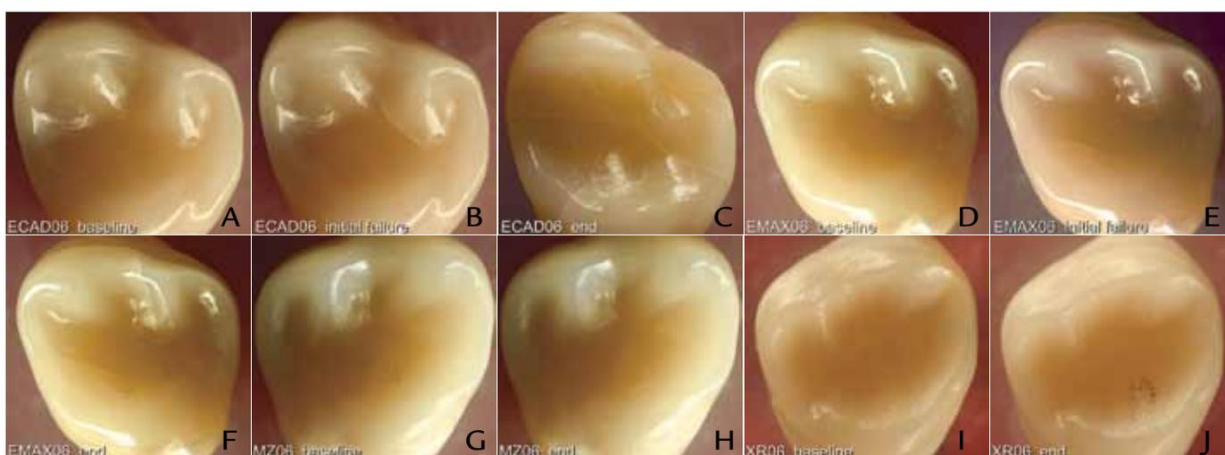
**5** A-C, Specimen in group ECAD. A, Before testing. B, At initial failure (400N). C, Lost fragment at 1400N. D-F, Specimen in group EMAX. D, Before testing. E, At initial failure (800N). F, After 185,000 cycles. G,H, Survived specimen in group MZ100. G, Before testing. H, After testing. I, J, Survived specimen in group XR. I, before testing. J, After testing.
