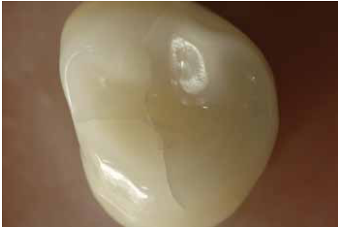
6 Specimen after testing in group ECAD. Note “mosaiclike” cracks.
