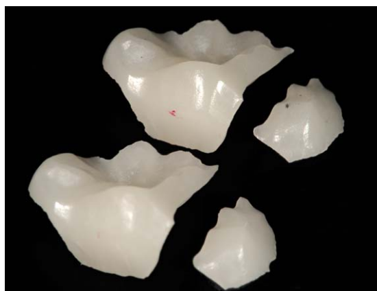
Fig. 4 – Onlay cusp overlap fracture.
