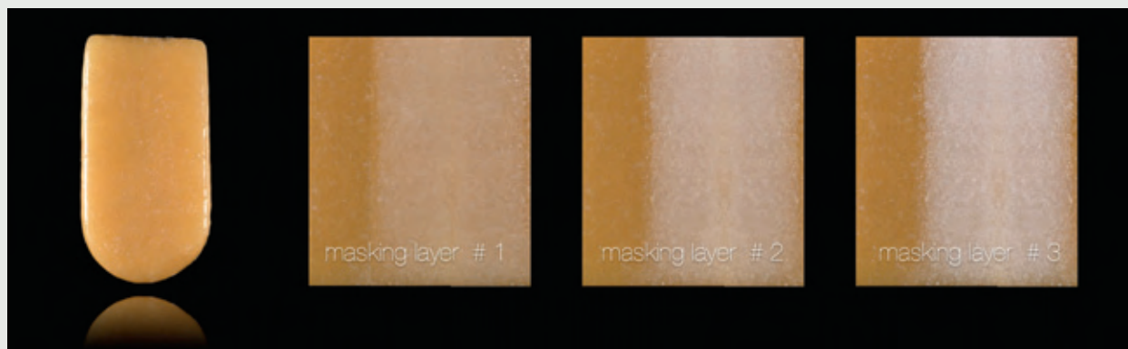
Fig 4 Sequential masking layers applied in the form of thin washes, where each layer is individually fired until the desired opacification of the test substrate is achieved.
