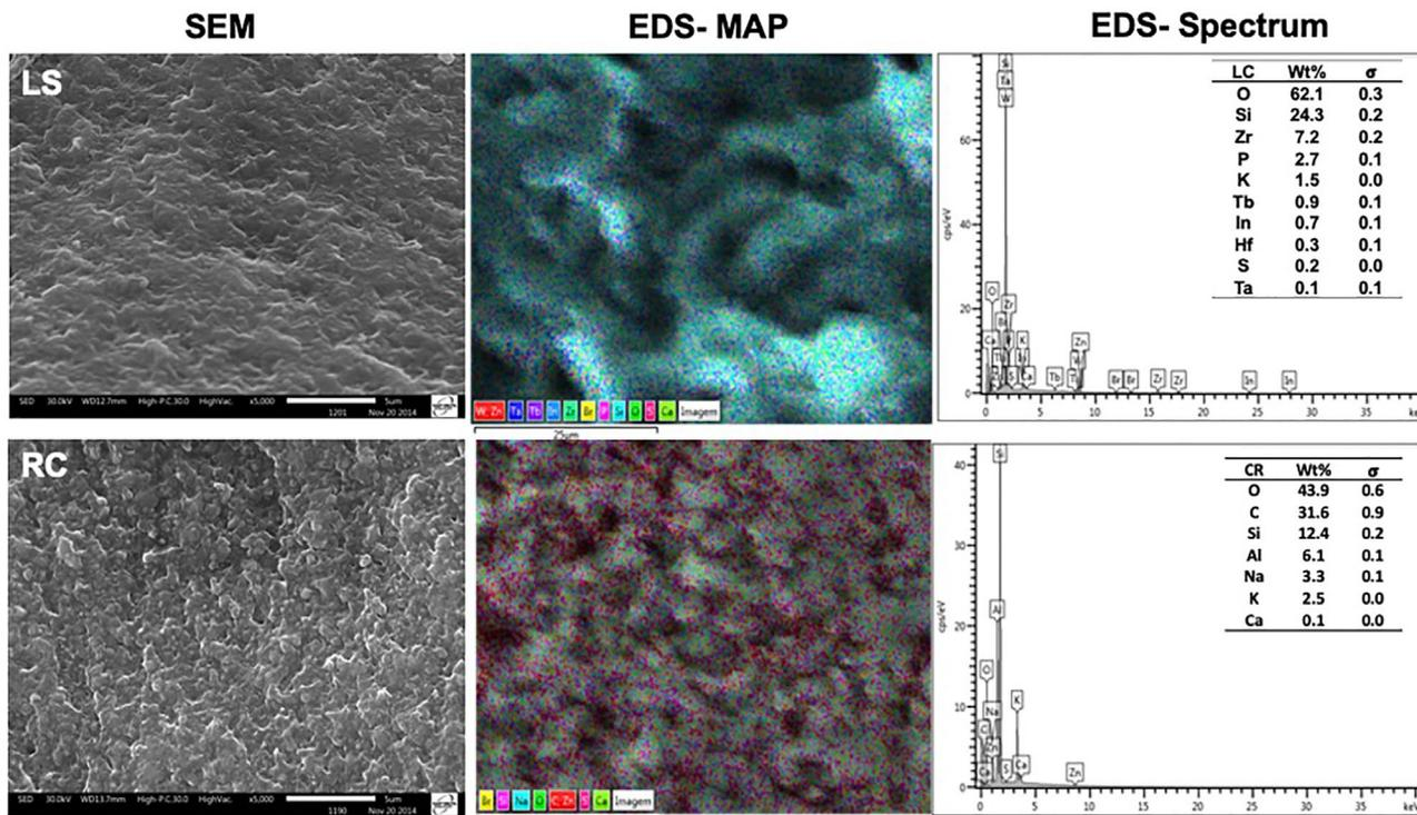
**FIGURE 6** SEM images (at 5000 $\times$  magnification) of CAD-CAM materials (left column), EDS mapping at 2000 $\times$  magnification, and EDS spectrum (right column). LS, lithium silicate and RC, resin-based composite.
