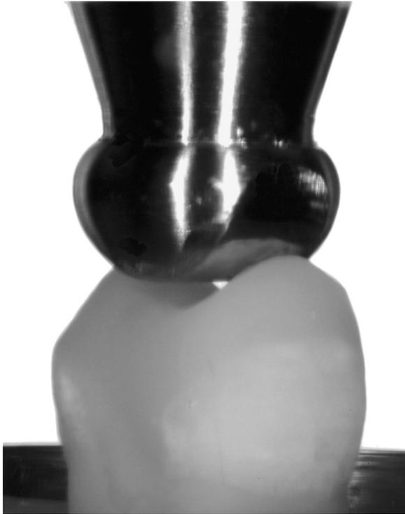
**Fig. 2 – Submerged specimen (2.5-mm overlap) in load chamber under isometric cyclic loading with stainless steel antagonist.**
