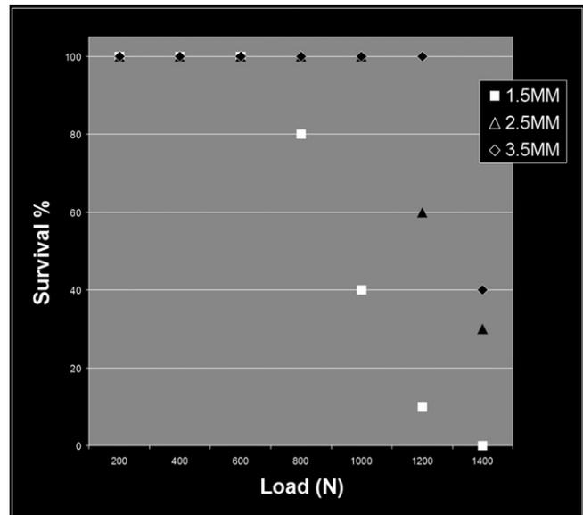
**Fig. 3 – Survival scatter plot of specimens at each load stage (n = 10).**
