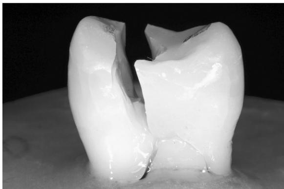
**Fig. 4 – Example of failed specimen (1.5-mm overlap) with fracture below CEJ (restoration and tooth).**
