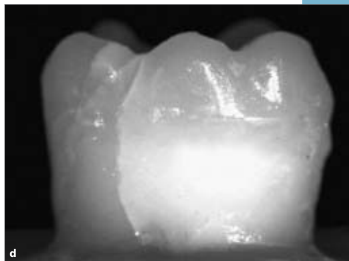
Figs 4a to 4d Examples of specimens. (a) Intact specimen in group M2. (b) Fracture above the CEJ in group M2; crack without fragment. (c) Fracture below the CEJ in group MKIIGL (a to c, original magnification \times 1.4 ). (d) Fracture below the CEJ without fragment in group MKIIGL-Z (original magnification \times 1.6 ).
