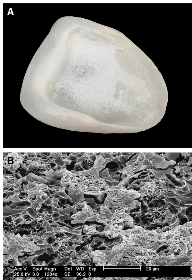
Fig. 2. A, Hydrofluoric acid etching of feldspathic porcelain typically generates white residue, contaminating etched surface, which may be confused with well-etched porcelain. B, SEM analysis (original magnification \times 1200 ) reveals that deposits may potentially prevent penetration of bonding resin into ceramic undercuts.
