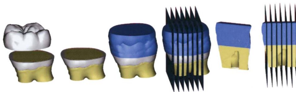
Fig. 2. Schematic representation of preparation of composite resin-dentin beams in “nontrimming” version of microtensile bond test.
